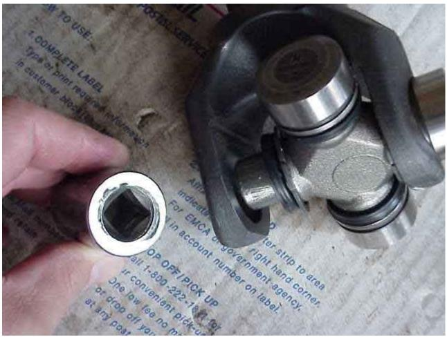
The solution was a Craftsman 7/8" half inch drive socket, as shown in the photo above. In this picture, I am just getting ready to push the bearing cap into the yoke (on the right side of the picture). I have slide the u-joint as far to the right as possible so that it is just into the needle bearings inside the bearing cap. (you don't want one of the bearings to fall over because you will have to take it all apart and do it over again....right after you almost got it all together!)
