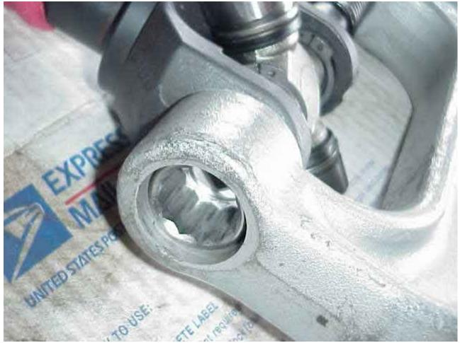
Here is a picture showing how well the socket keeps the HF tool centered in position. Keeping things aligned like this when tightening the screw on the u-joint tool goes a long way in making this entire task just a bit easier.
